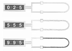
In this diagram, a standard ER instrument is connected to a 40 mil wire loop element which has a useful life of 10 mils. The instrument still reads close to zero because the element is new.
